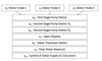
Figure 3: Diagram of water supply subsystem in the form of a directed graph
