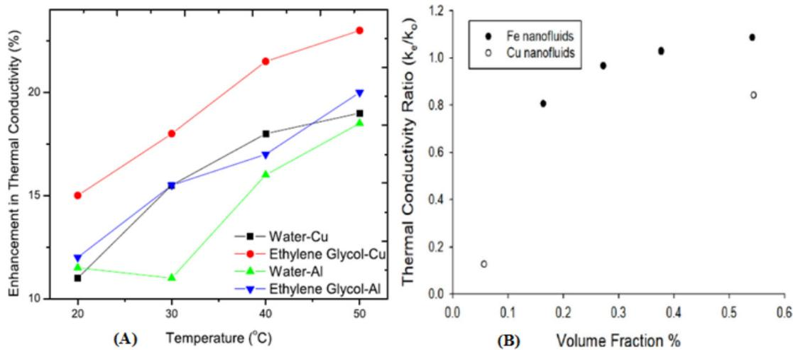
Figure 5: (A) The relationship between Cu and Al with different base fluids and enhancement in thermal energy, (B) The relationship between volume fraction and the thermal conductivity of Fe and Cu nanofluids [74]
