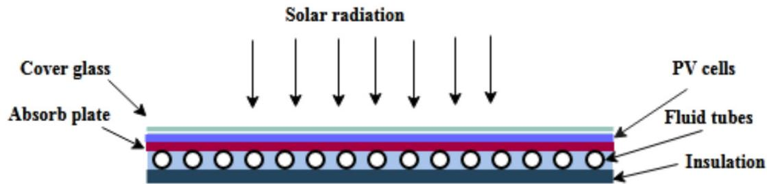
Figure 1: Schematic diagram of the hybrid PV/T system
