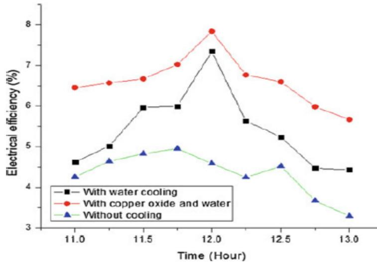
Figure 8: The behavior of the electrical efficiency with and without cooling
