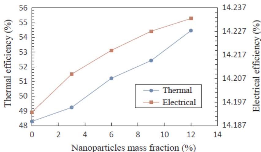
Figure 9: The effect of nanoparticles mass fraction on the efficiency of the PV/T system
