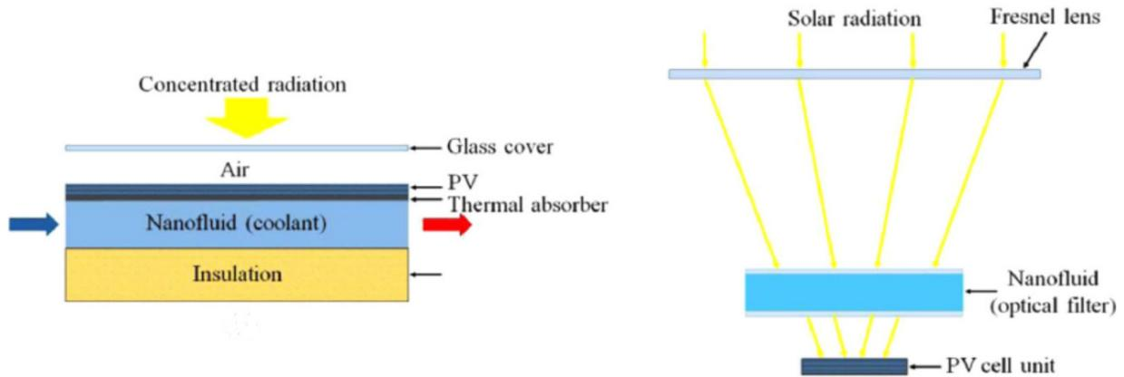
Figure 3: Schematic of the PV/T system with nanofluid as a coolant and spectral [60]
