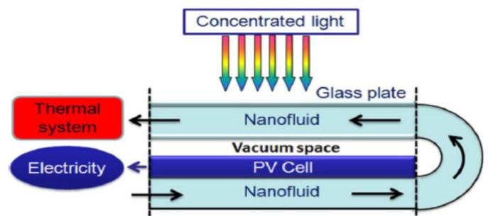
Figure 6: Decoupled PV/T system use nanofluid as a working fluid
