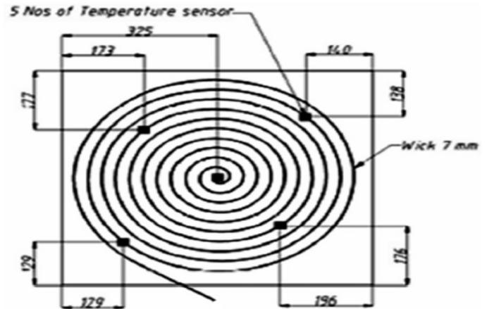
Figure 10: Cotton wick structures fixed in the back of the PV
