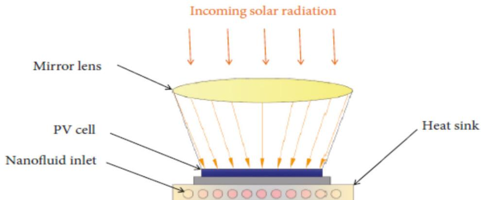
Figure 4: Schematic diagram of the CPV/T system work on nanofluid [64]
