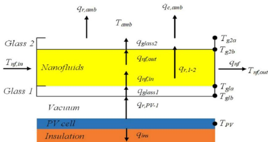
Figure 7: Schematic diagram of using optical filtration nanofluid for the PV/T system
