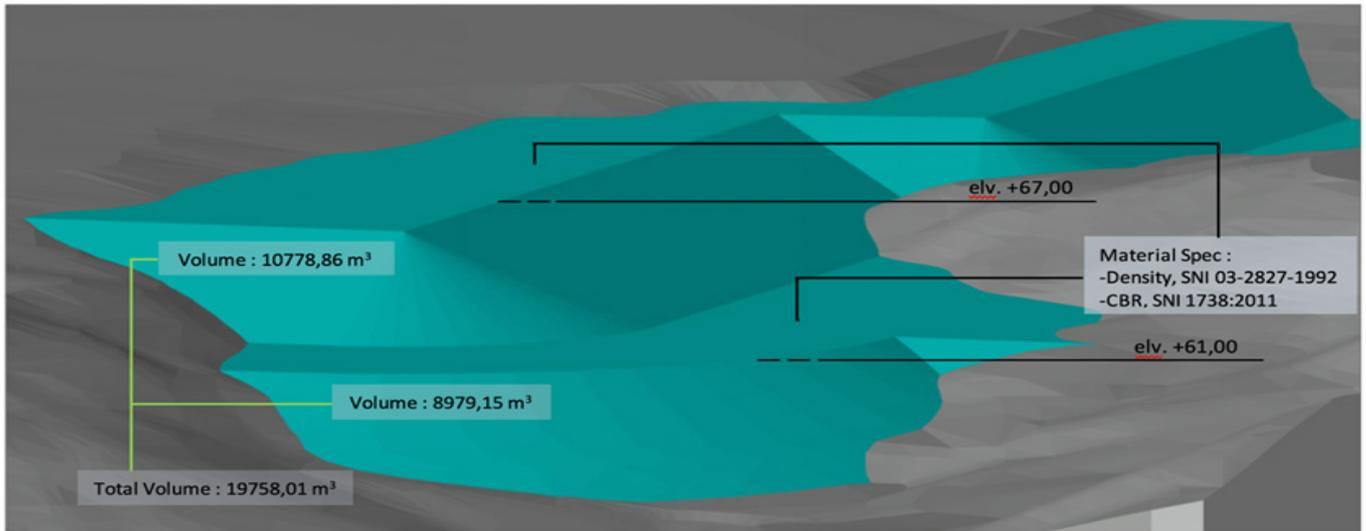
Figure 10: Final design for slope in 3D visualization
