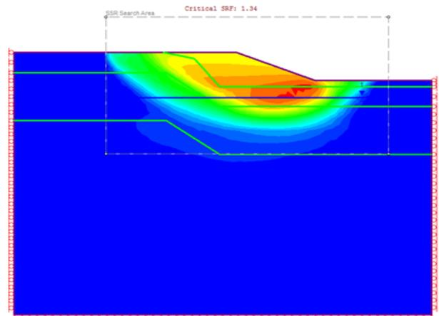
Figure 8: Two-dimensional numerical analysis result for section A-A in dynamic condition
