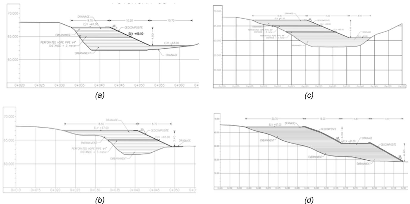
Figure 9: Geometry for slope after countermeasures applied (a) Section A-A (b) Section B-B (c) Section C-C (d) Section D-D
