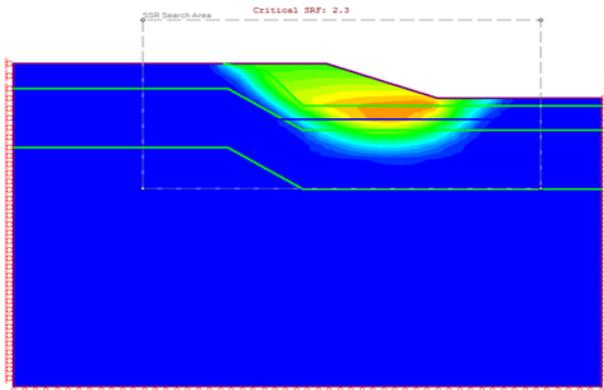
Figure 7: Two-dimensional numerical analysis result for section A-A in static condition
