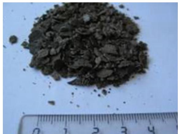
Figure 1: Appearance of scale from well No. 14096
