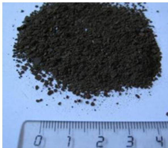
Figure 3: Appearance of scale from well No. 19617
