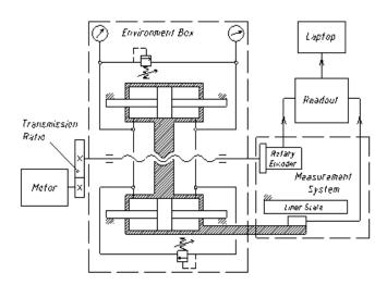
Figure 1: Overall diagram of experiment machine
