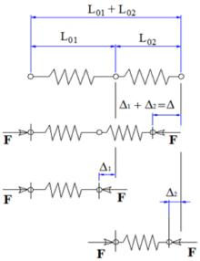
Figure 2: Relationship between axial wear and deviation: L02 – the amount of wear ( $\mu$ m); L01 – the length left after wear ( $\mu$ m); F – the axial load (N);  $\Delta_1$  – the amount of elastic deformation of L<sub>01</sub> ( $\mu$ m);  $\Delta_2$  – the amount of elastic deformation of L<sub>02</sub> ( $\mu$ m);  $\Delta$  - the elastic deformation before wear ( $\mu$ m)
