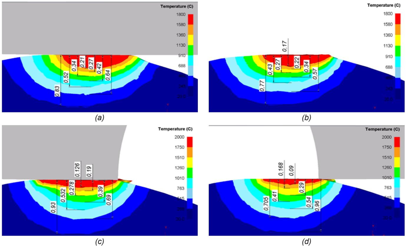
Figure 6: Models of temperature change in one revolution of the disk in the heating and cooling zones, with  $L_1=26$  mm;  $L_2=6$  mm (a,b -  $n_0=2000$  r/min; c,d -  $n_0=3000$  r/min;  $S=120$  mm/min;  $e=2$  mm; a,c – models of heating zone  $L_1=26$  mm; b,d – models of cooling zone  $L_2=6$  mm)
