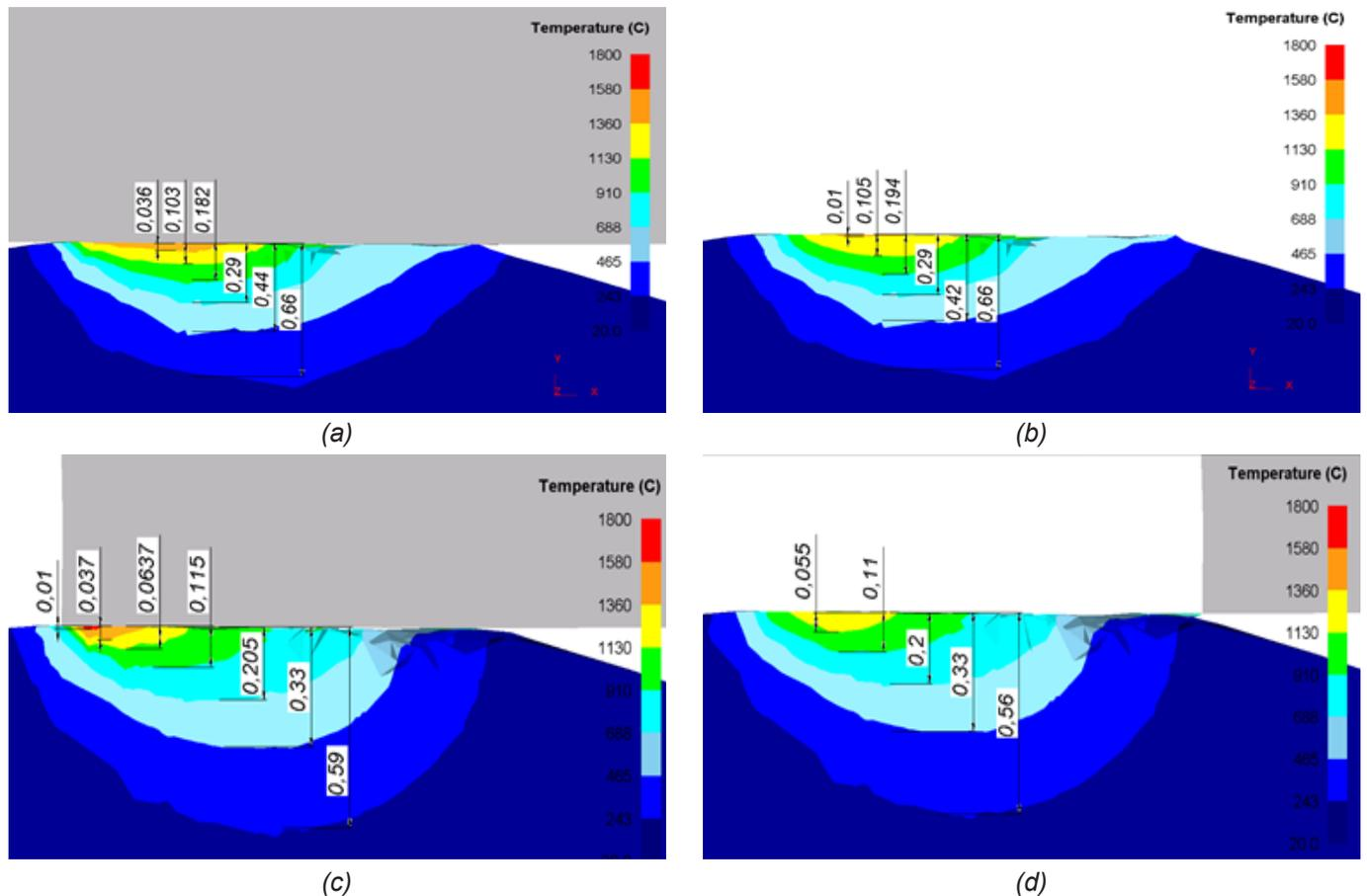
Figure 5: Models of temperature change in one revolution of the disk in the heating and cooling zones, with  $L_1=18$  mm;  $L_2=14$  mm (a,b -  $n_\theta=2000$  r/min; c,d -  $n_\theta=3000$  r/min;  $S = 120$  mm/min;  $\delta = 2$  mm; a,c – heating zone models  $L_1=18$  mm; b,d – cooling zone models  $L_2 =14$  mm)
