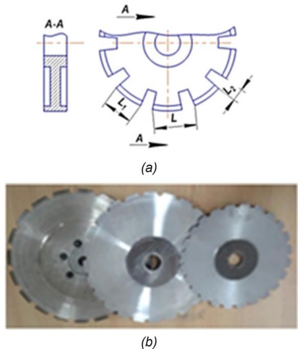
Figure 1: Sketch and photos of a special circular saw (a - sketch of a circular saw; b - photos of circular saws; L - tooth pitch; L<sub>1</sub> - heating zone; L<sub>2</sub> - cooling zone)
