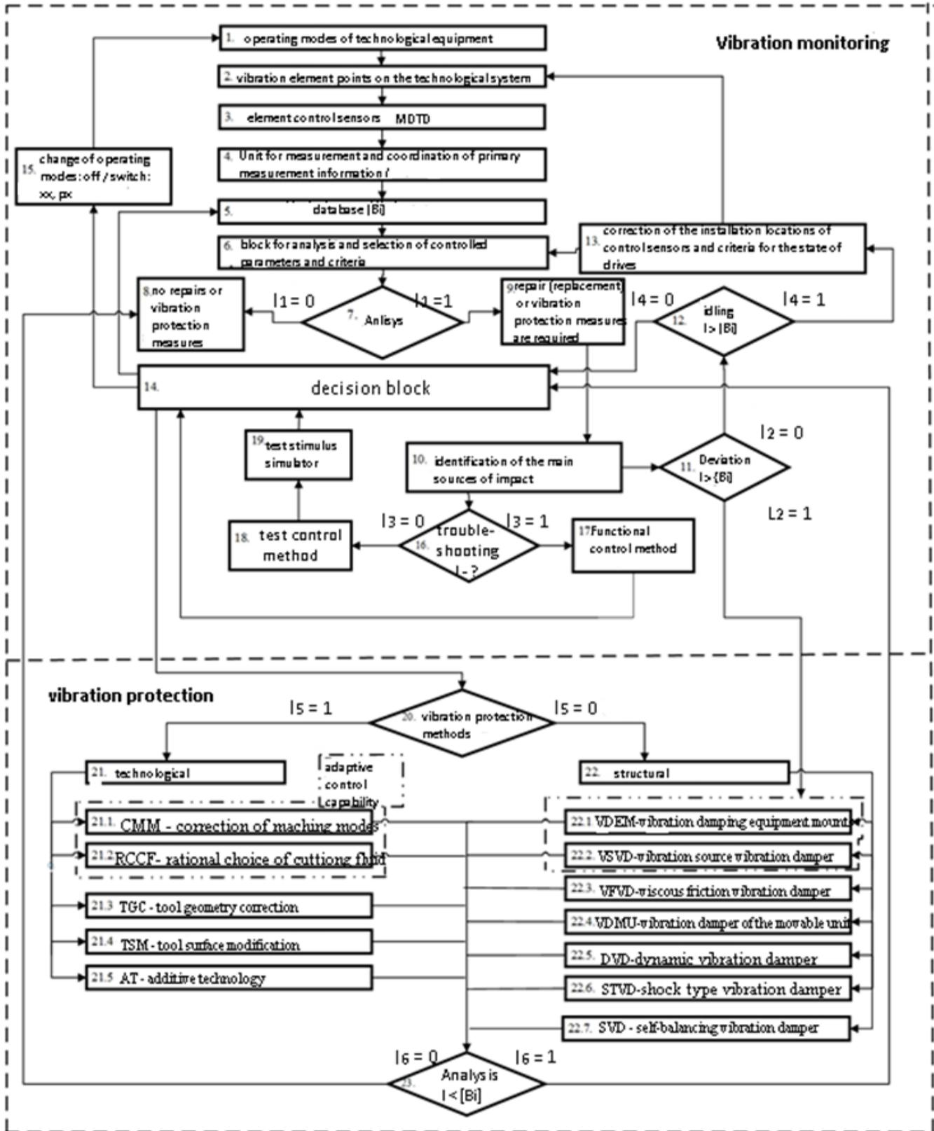
Figure 3: Block diagram of the algorithm for the selection and rational use of structural and technological methods of vibration protection of vehicle elements in order to increase the efficiency of machining based on the results of functional and test vibration monitoring (Ij-bits of information)
