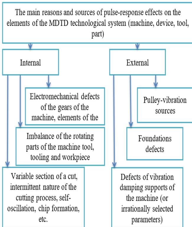
Figure 1: The main causes and sources of impulse - vibration effects on MDTD elements
