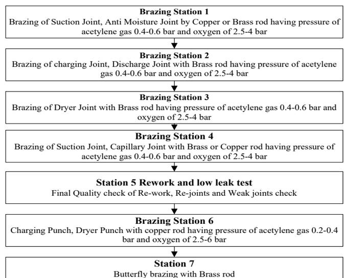
Figure 3: Flow process map of Brazing process
