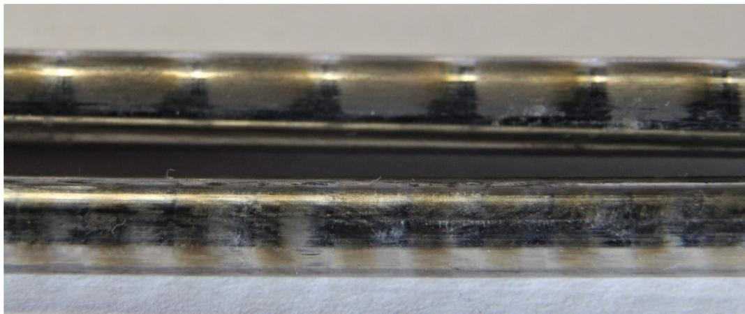
Figure 2: Appearance of the defect "heterogeneity"
