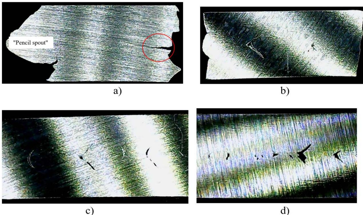
Figure 4: a - "Pencil spout" (red ovals are highlighted in cracks in the metal); b - A view of "crow's feet" at a distance of 75 mm from the breakage point (from the spout of the "pencil"); c - A view of "crow's feet" from the opposite end of the sample from the breakage point (sample with the spout of the "pencil"); d- A view of "crow's feet" and cavities from the opposite end of the second sample from the breakage point
