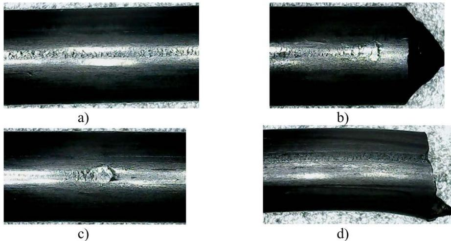
Figure 3: Samples for the study: a - The general nature of the flaws on the samples; b - The view of the flaws at the place of the break on one of the samples; c - A flaw 75 mm from the place of the break on the sample; d- Flaws on the response sample
