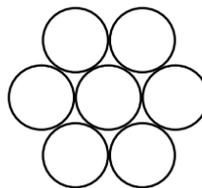
Figure 1: Cross section of a seven-wire reinforcing rope structure
