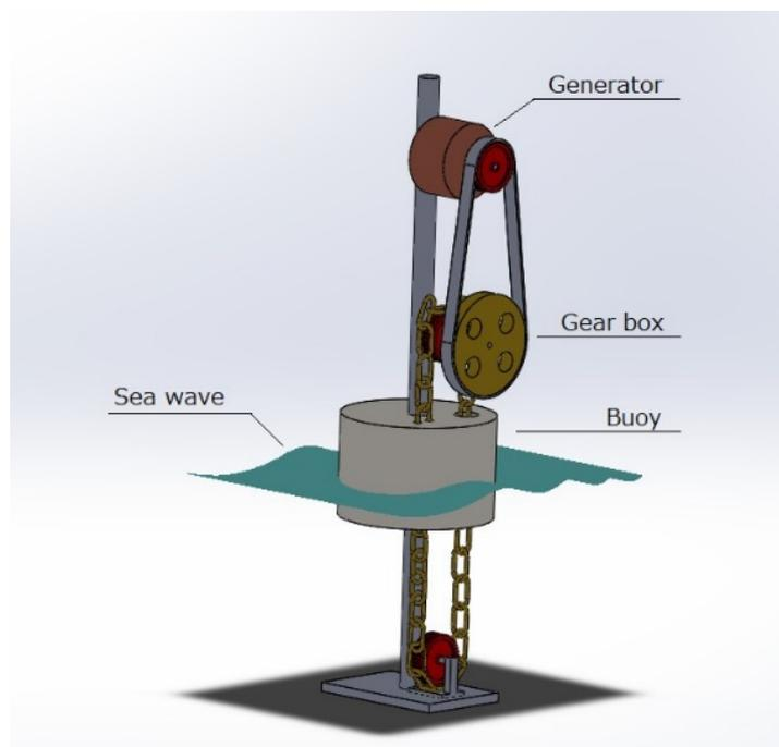
Fig. 3. Electric generation system from waves energy
