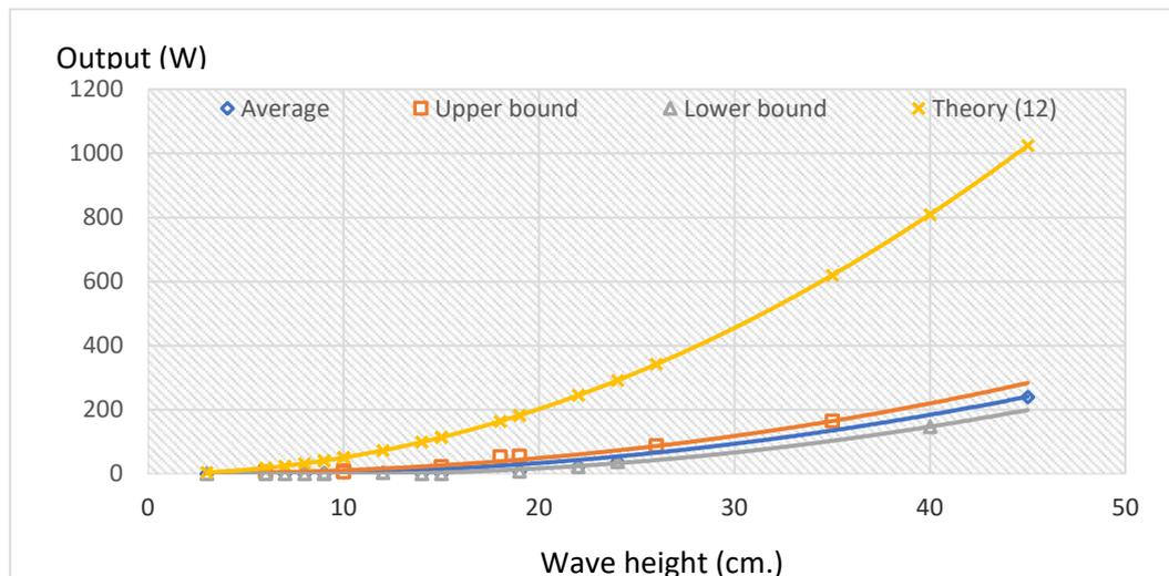
Fig. 5. Output power of the generator
