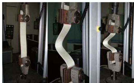
Fig. 4. Buckling process and deformation shape of a laminated composite plate during compression test
