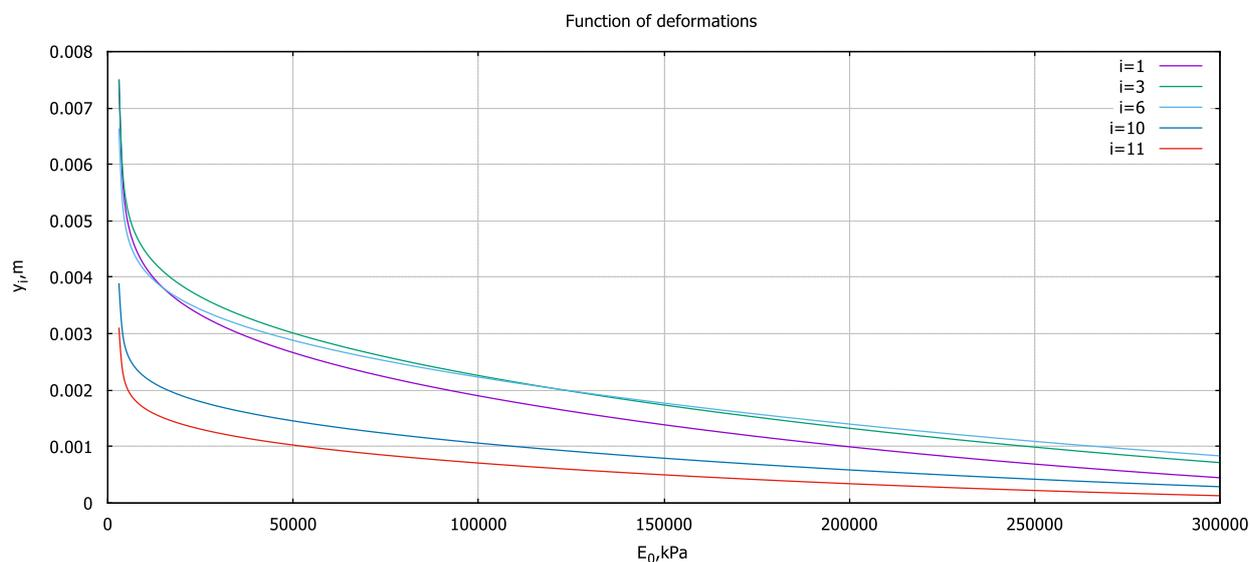
Figure 6. Dependence of a beam lying on an elastic foundation deflection on the values of the foundation material deformation modulus
