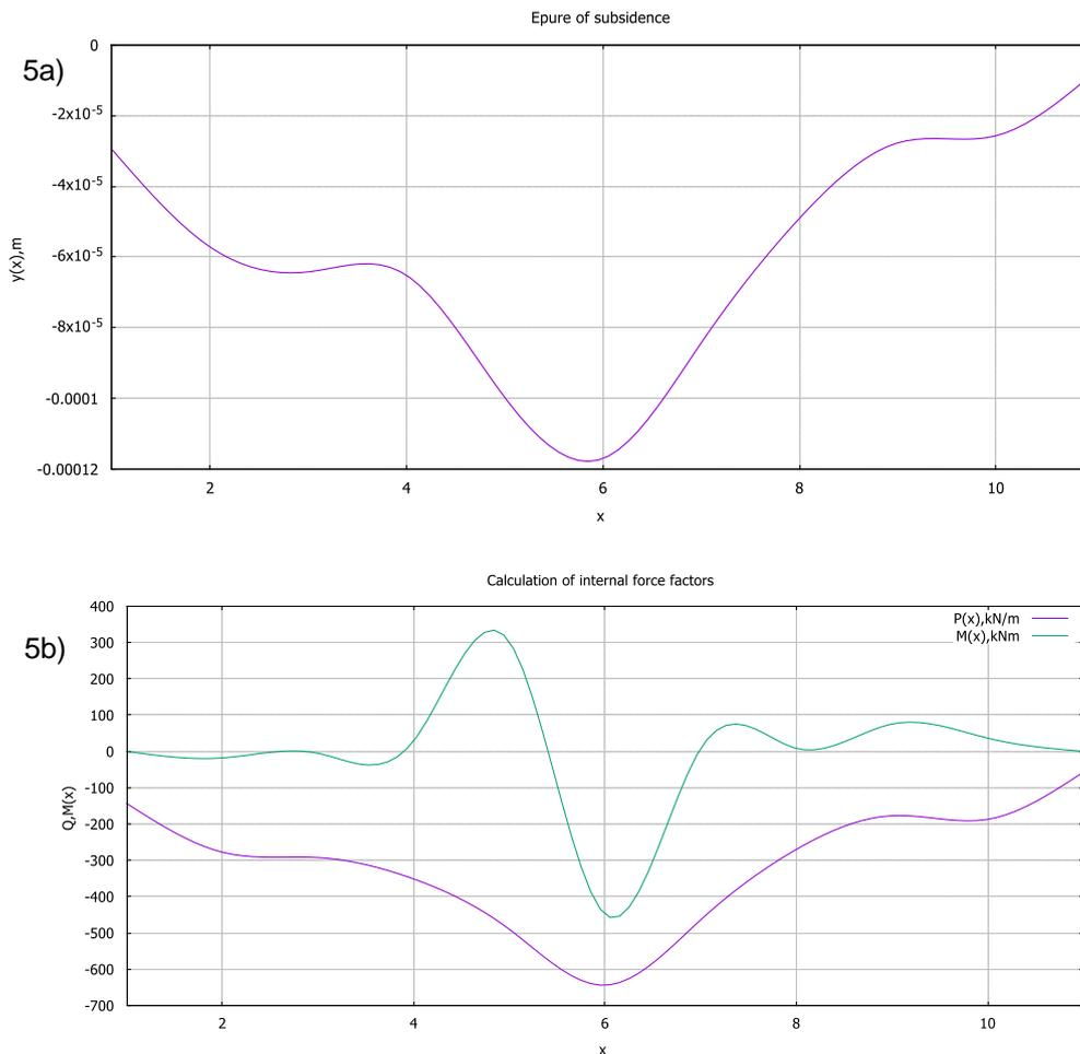
Figure 5: The results of designing the beam in Fig. 1
