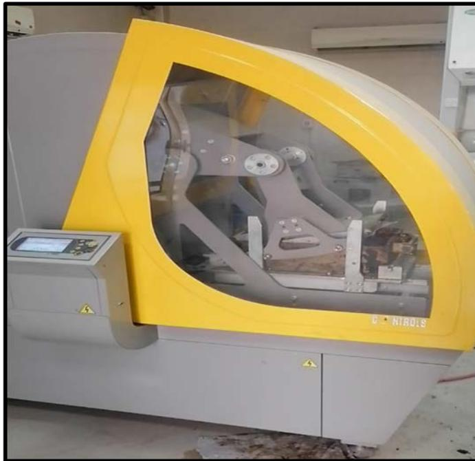
(a) Compacting the sample by roller compactor.
