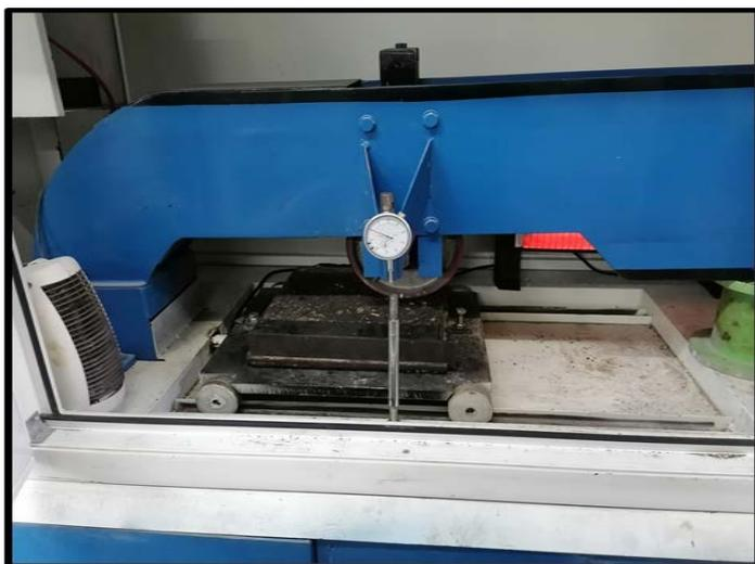
(c) Slab inside wheel tracking machine.
