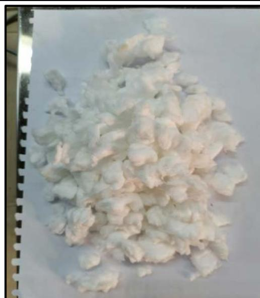
Figure 2. The appearance of ceramic fiber
