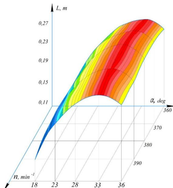
Fig. 5. Helix angle elevation  $\alpha$  and screw feeder speed  $n$  (at  $V_{per}=0.3s^{-1}$ ;  $h=0.1m$ ) affecting the snow mass throwing distance
