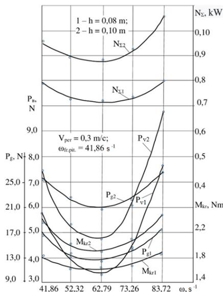
Fig. 9. Influence of the rotation speed of the bladed intensifier  $\omega$  on the torque  $M_{kr}$ , total power  $N_{\Sigma}$ , vertical  $P_v$  and horizontal  $P_g$  forces: 1)  $h = 0.08\text{ m}$ ; 2)  $h = 0.10\text{ m}$
