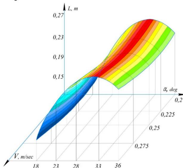
Fig. 4. Helix angle rise  $\alpha$  and operating speed  $V$  (at  $n=400 \text{ min}^{-1}$ ;  $h=0.1 \text{ m}$ ) affecting the snow mass throwing distance
