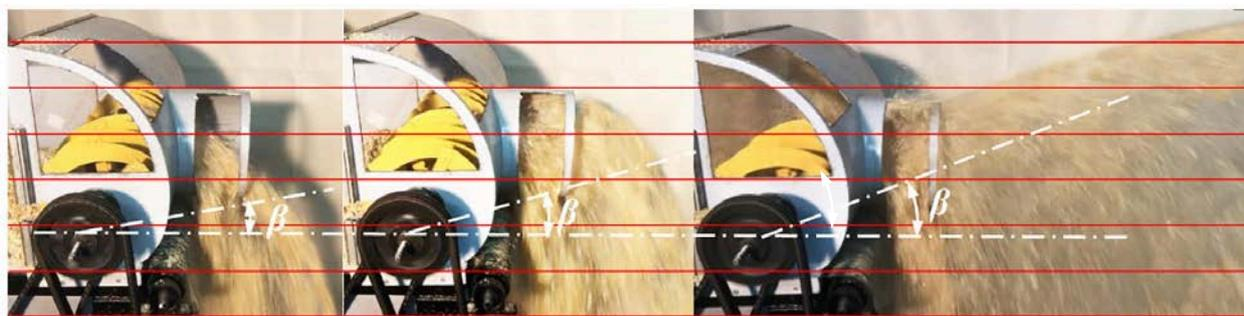
Fig. 6. Photograph of the material ejection process by a milling feeder into the conditional area of operation of the rotor-thrasher with the angle of helix elevation: 1)  $\alpha=38^{\circ}$ ; 2)  $\alpha=28^{\circ}$ ; 3)  $\alpha=18^{\circ}$
