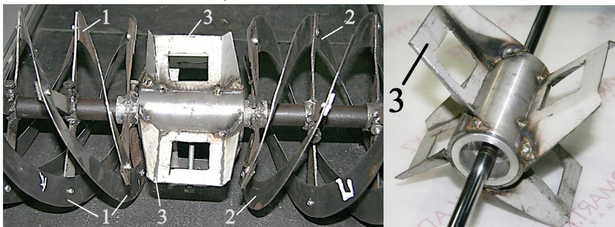
Fig.1. Scheme of the FRS screw feeder: 1 - left semi-mill; 2 - right semi-cut; 3 - bladed intensifier
