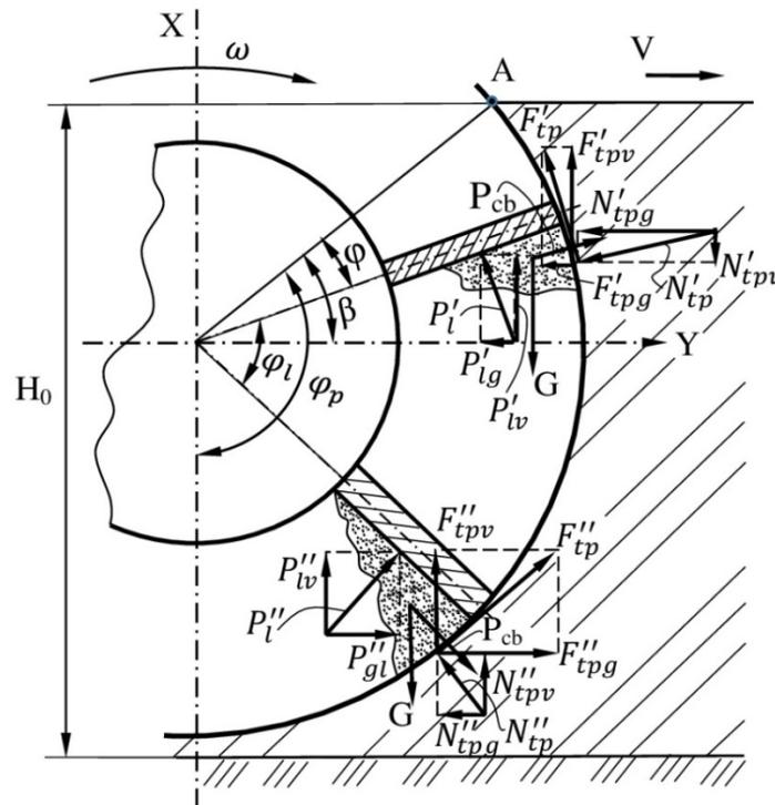
Figure 2 - Forces applied to the intensifier blades
