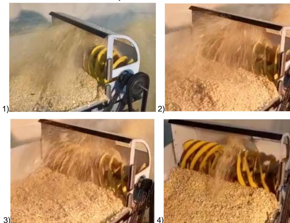
Fig. 7. Photograph of the process of throwing forward a mass of material simulating snow by a milling feeder:
