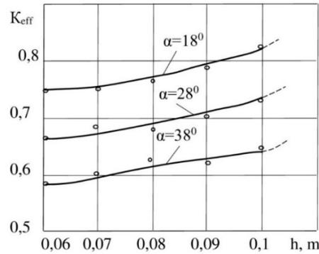
Fig. 8. Influence of the helix angle  $\alpha$  and the height of the developed snow  $h$  on the efficiency coefficient  $K_{eff}$
