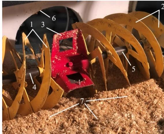
Fig. 3. Physical model of the MRS with a paddle intensifier, mounted on an experimental stand to study the working processes of snowplows
