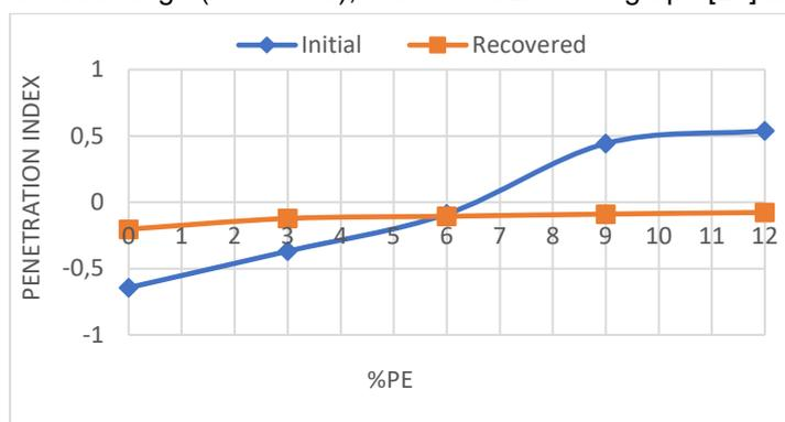
Fig. 4. Penetration index of PESA
