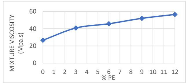
Fig. 7. PESAM extensional viscosity.
