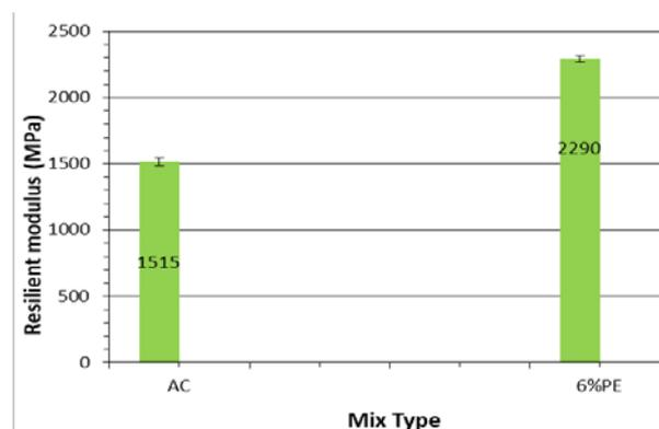
Fig. 12. Resilient modulus of AC and PEAC mixtures.
