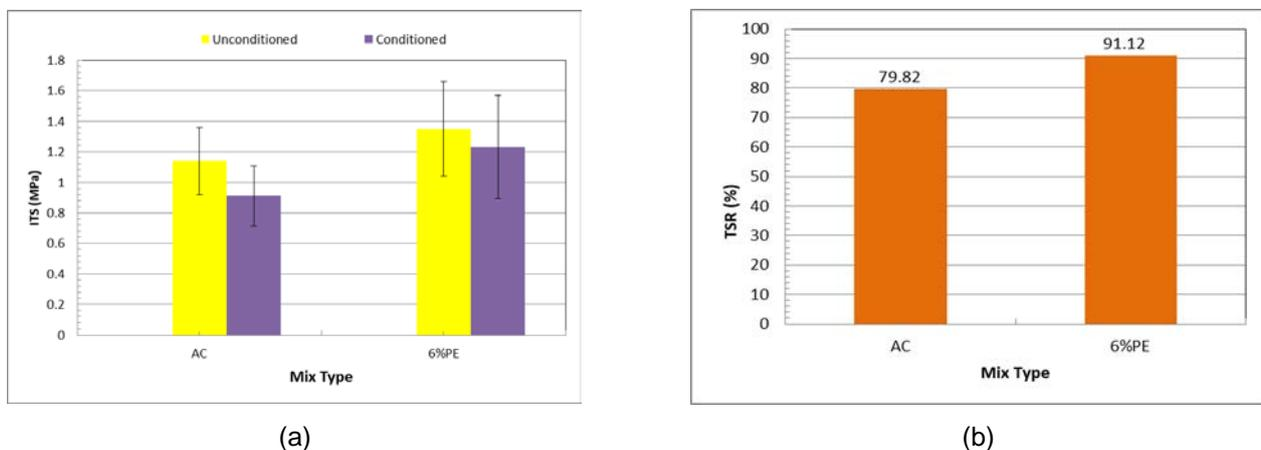
Fig. 11. Properties of indirect tensile strength in mixes of AC and PEAC
