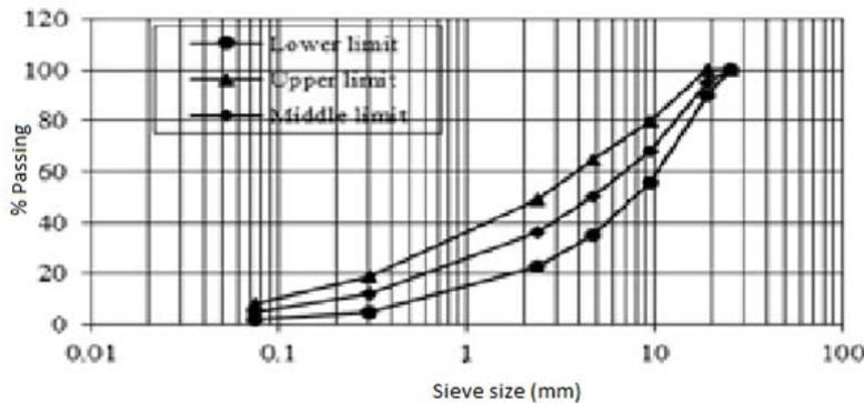
Fig. 2. Aggregate gradation
