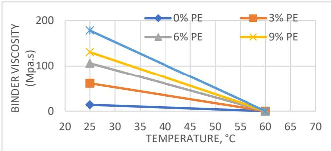
Fig. 8. PESA Viscosity at extension at 25 and 60 °C
