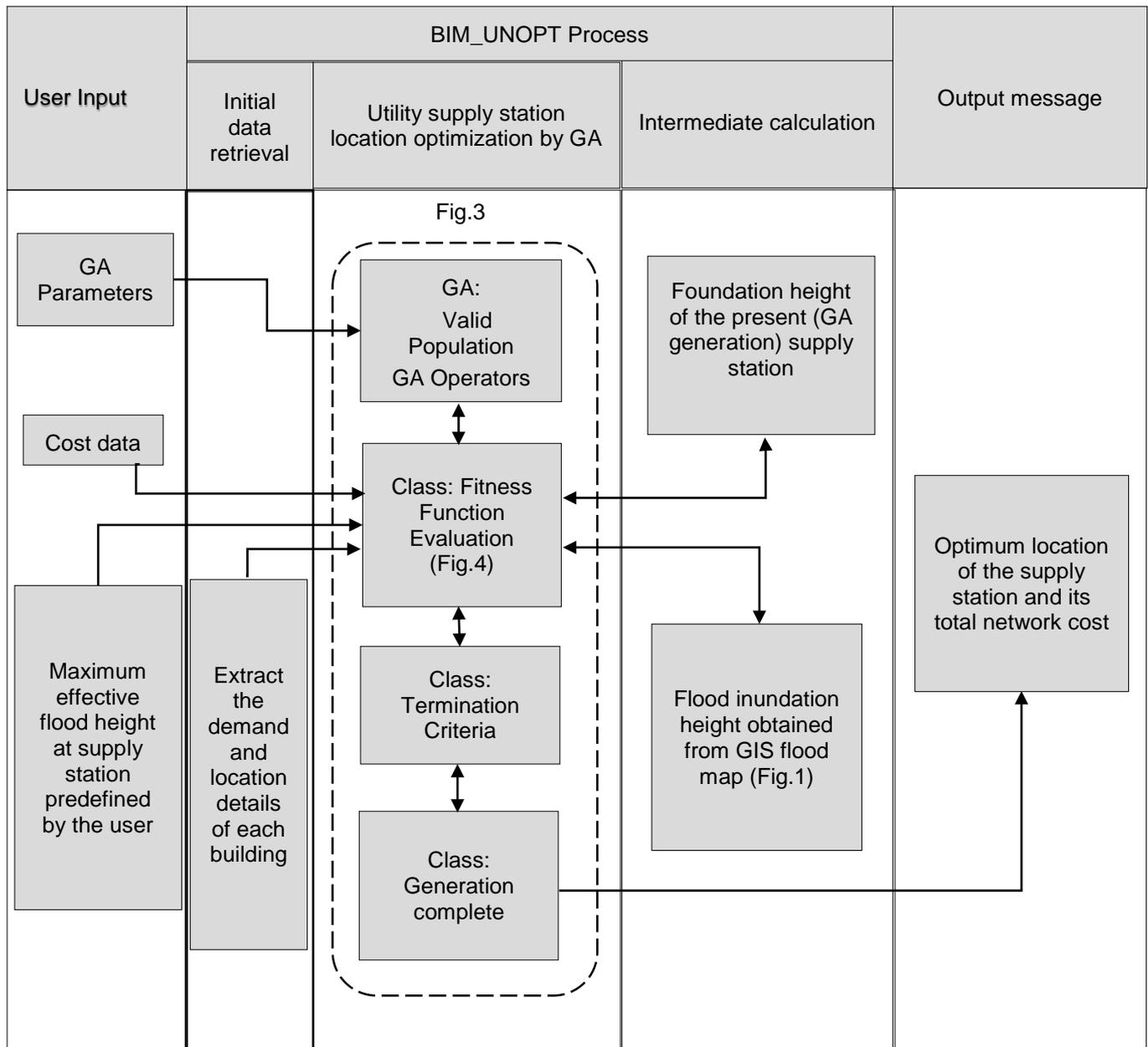
Fig. 2. Information flow diagram for utility supply station location optimization
