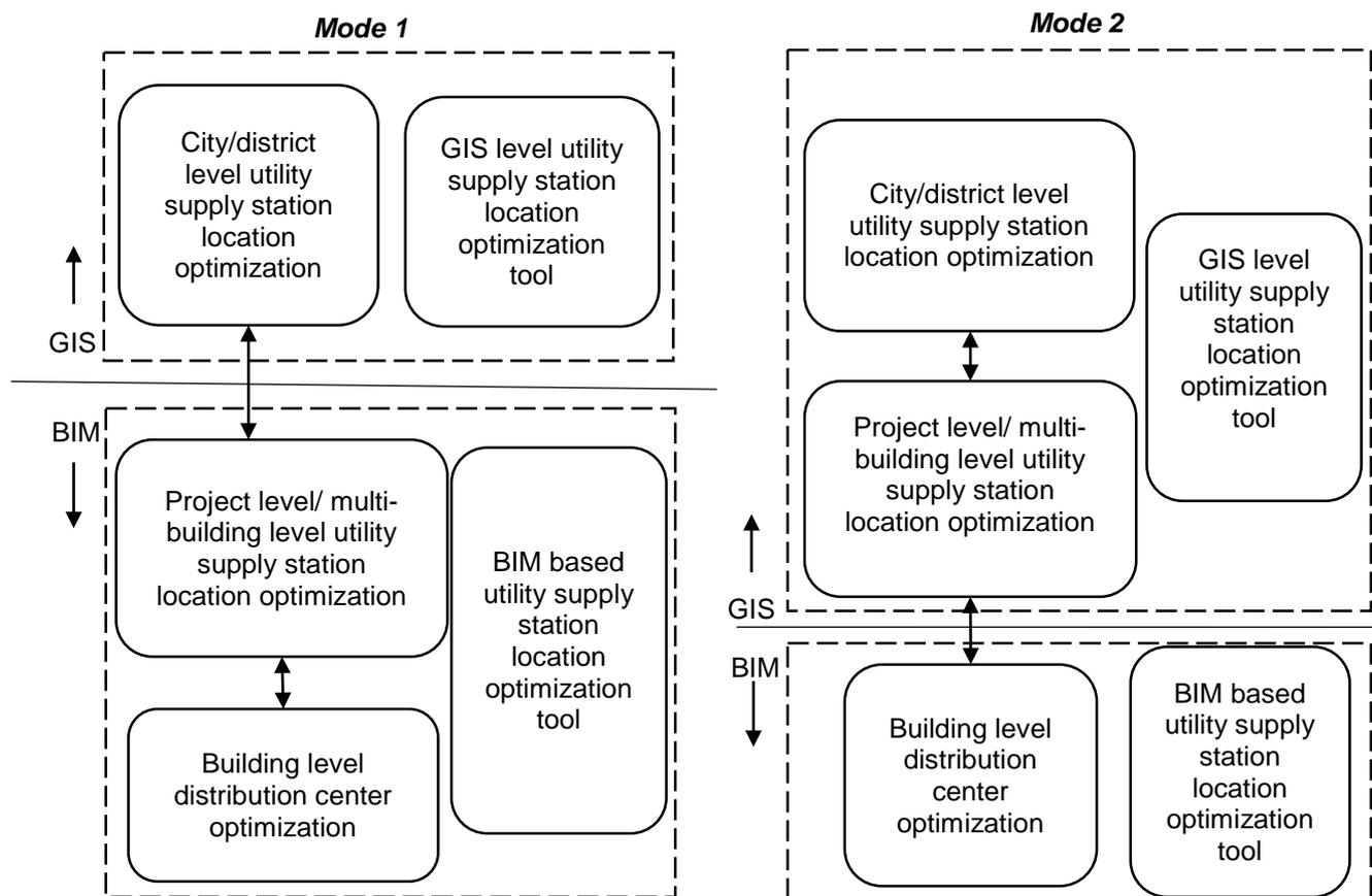
Fig. 9. Two mode of BIM-GIS integration for multi-stage utility supply station location optimization
