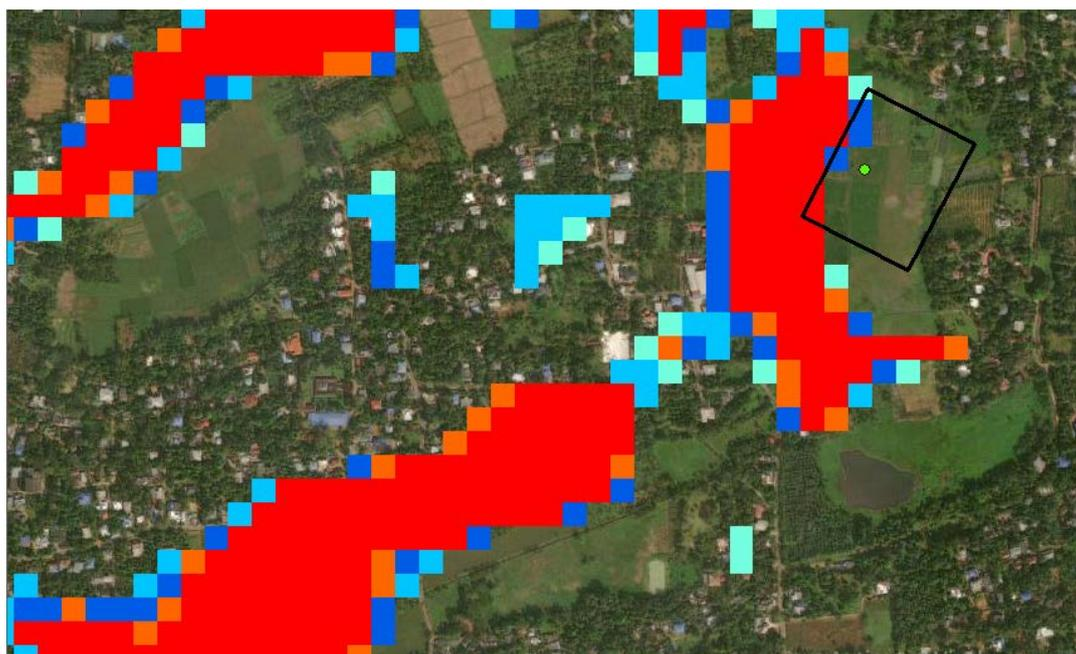
Fig. 5. The flood inundation height raster data with google map background for the location of the case study. The black hollow rectangle area is the project site
