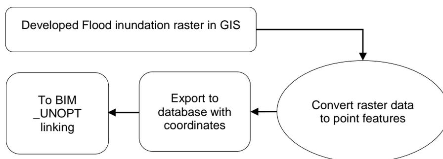
Fig.1. Flow chart of flood GIS data conversion to BIM
