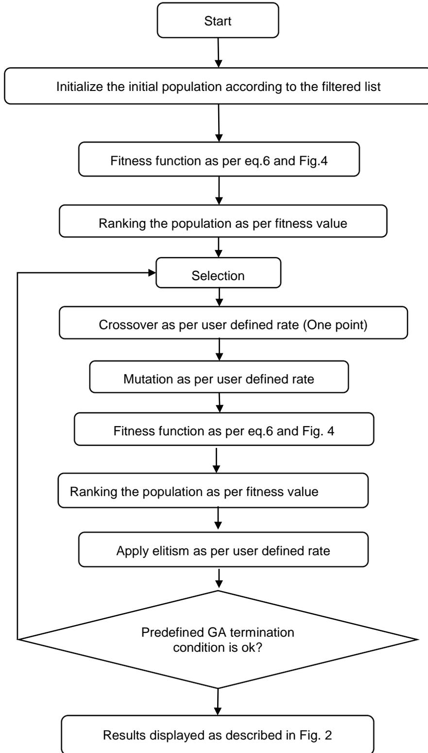
Fig. 3. Flowchart for GA process
