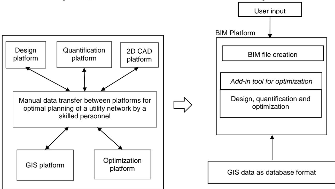
Fig. 8. The conventional and the proposed process of utility supply station location optimization
