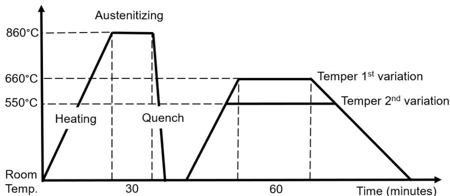
Fig. 3. Heat treatment procedure
