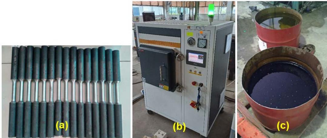
Fig. 2. Test specimens and setup equipment: (a) ASTM E8 specimens; (b) electric furnace; (c) quench media
