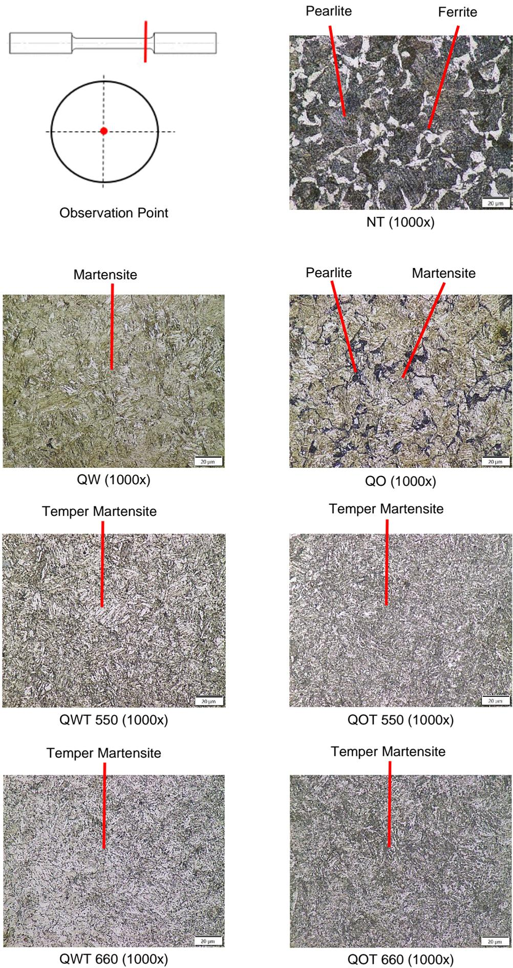
Fig. 7. Metallography of the core region of the specimen
