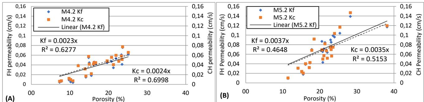
Fig. 8. The correlation between the porosity and permeability coefficient of PCM is measured by the constant head and falling head method at (A) S/C 4.2 and (B) S/C 5.2
