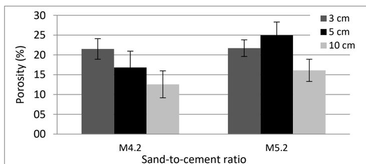
Fig. 2. Effect of sand-to-cement ratio and thickness on its porosity
