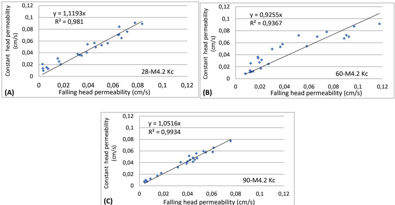
Fig. 5. Correlation of PCM permeability measured by the constant head and falling head method (S/C 4.2) in different ages (A) 28 days, (B) 60 days, and (C) 90 days
