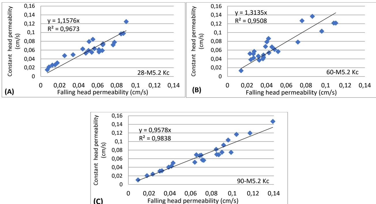
Fig. 6. Correlation of PCM permeability measured by the constant head and falling head method (S/C 5.2) in different ages (A) 28 days, (B) 60 days, and (C) 90 days
