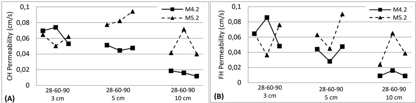
Fig. 4. Permeability coefficient at different ages of specimens and thickness by (A) constant head and (B) falling head method
