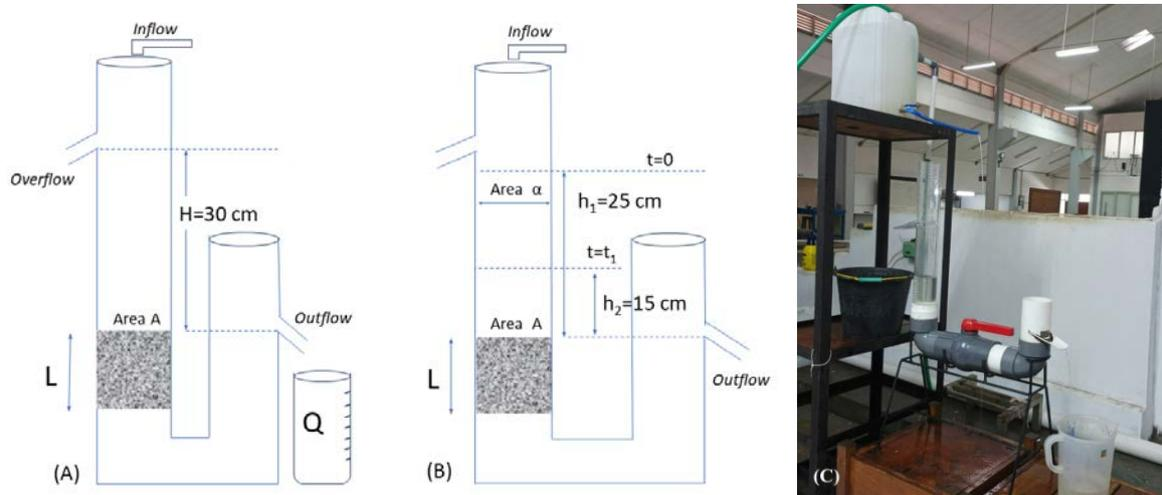
Fig. 1. The scheme of permeability coefficient calculation (A) constant head method, (B) falling head method, and (C) Permeability test apparatus for both constant head and falling head method
