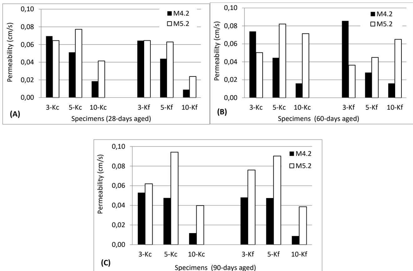
Fig. 3. Permeability coefficient at different S/C ratios and thicknesses at the age of (A) 28 days, (B) 60 days, and (C) 90 days
