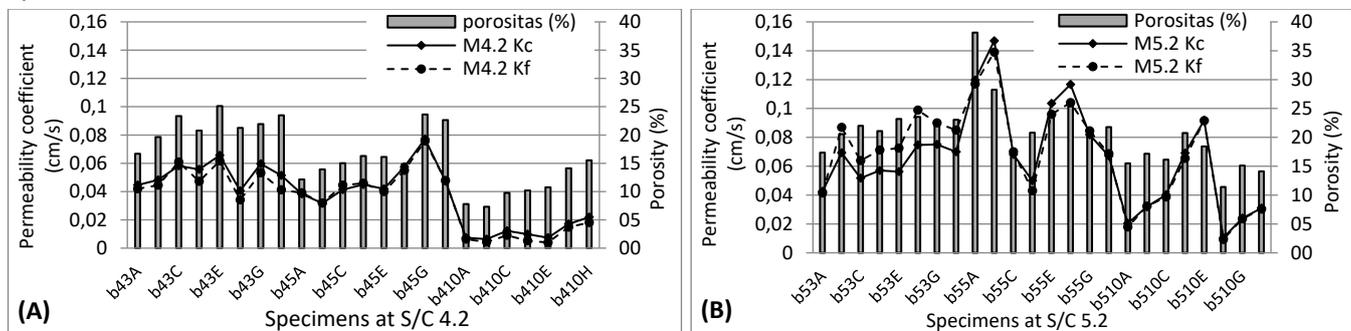
Fig. 7. Relationship of permeability and porosity of PCM specimens at (A) S/C 4.2 and (B) S/C 5.2
