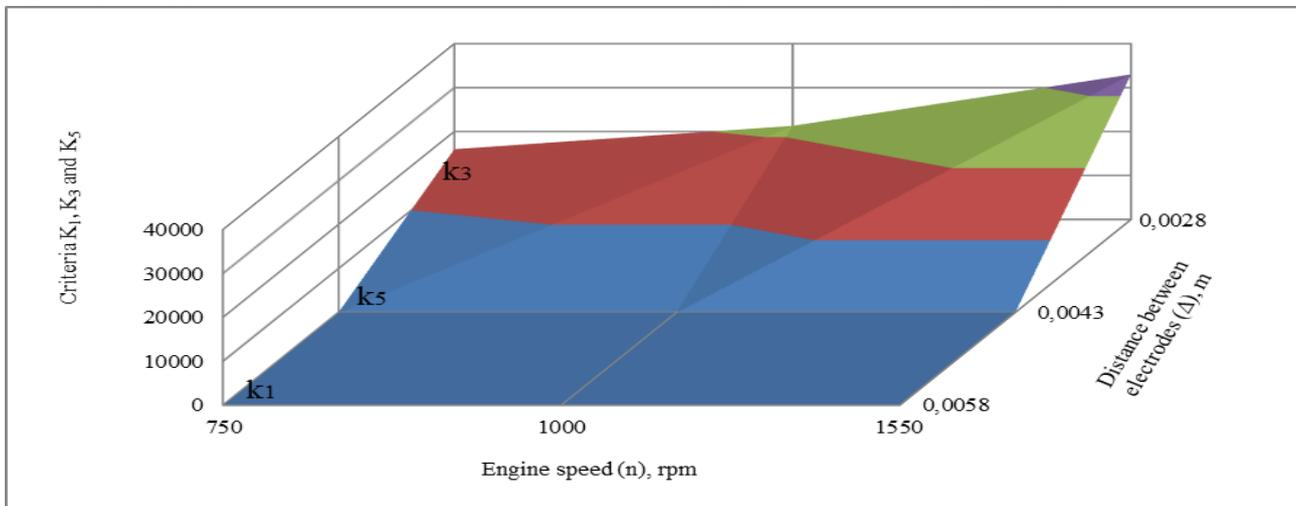
Fig. 9. Graph of dependencies of criteria  $k_1$  and  $k_3$  on changes in engine speed ( $n$ ) and distances between electrodes ( $\Delta$ )
