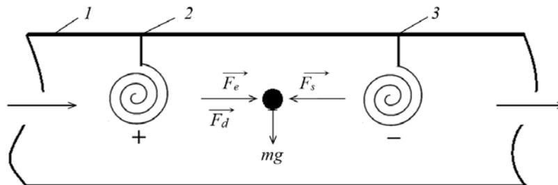
Fig. 5. Diagram of the forces acting on a gas particle in the muffler
