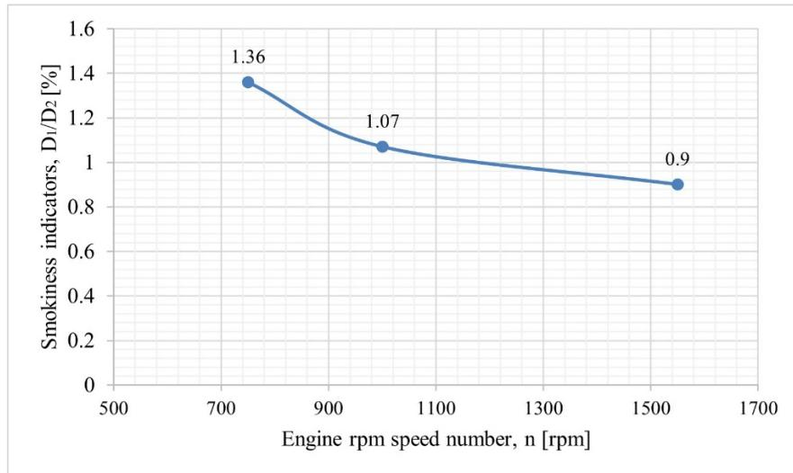
Fig. 8. Graph of the dependences of the optimality criterion on the change in engine speed  $n$
