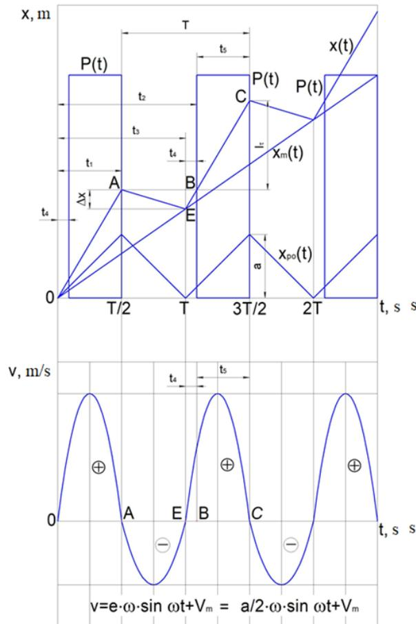
Fig. 4. Mechanism of vibrational cutting (trajectory of the cutting-edge movement, velocity of the cutting edge, cutting force impulses)
