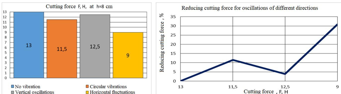
Fig. 12. Influence of the direction of vibrations on the magnitude of cutting force
