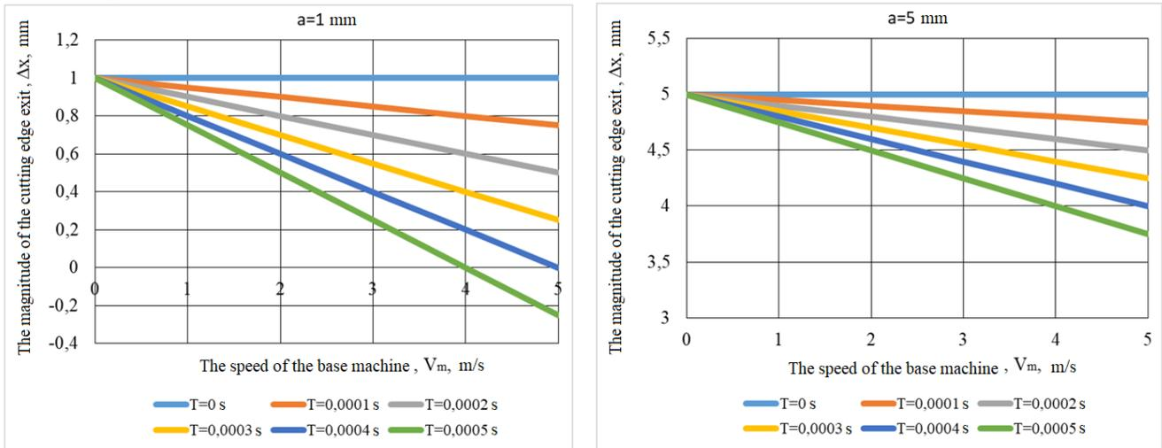
Fig. 5. Influence of the movement speed of the base chassis  $V_m$  on the magnitude  $\Delta x$
