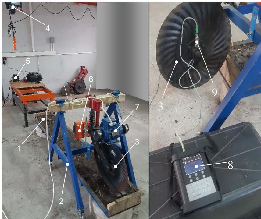
Fig. 11. Experimental stand for studying vibrational disc working organs of seeders
