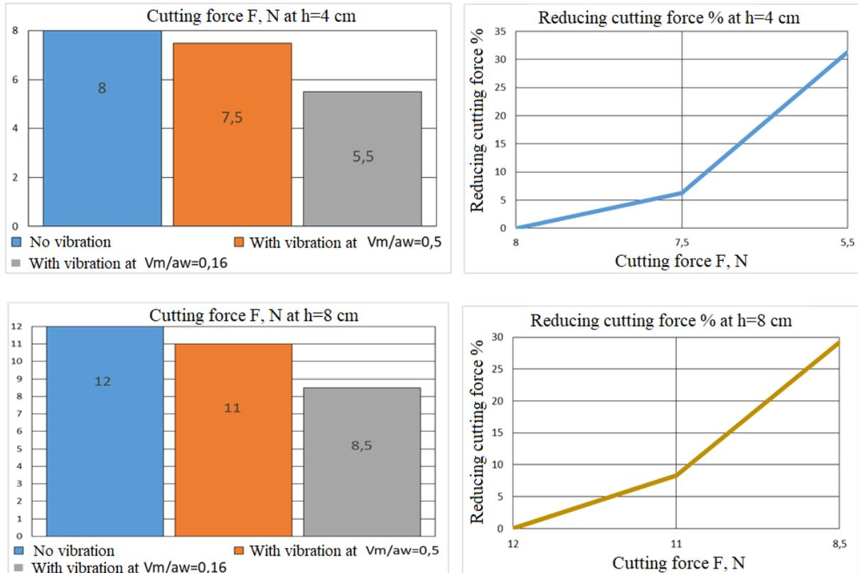
Fig. 13. Cutting force as a function of the parameter  $\frac{V_m}{a \cdot \omega}$
