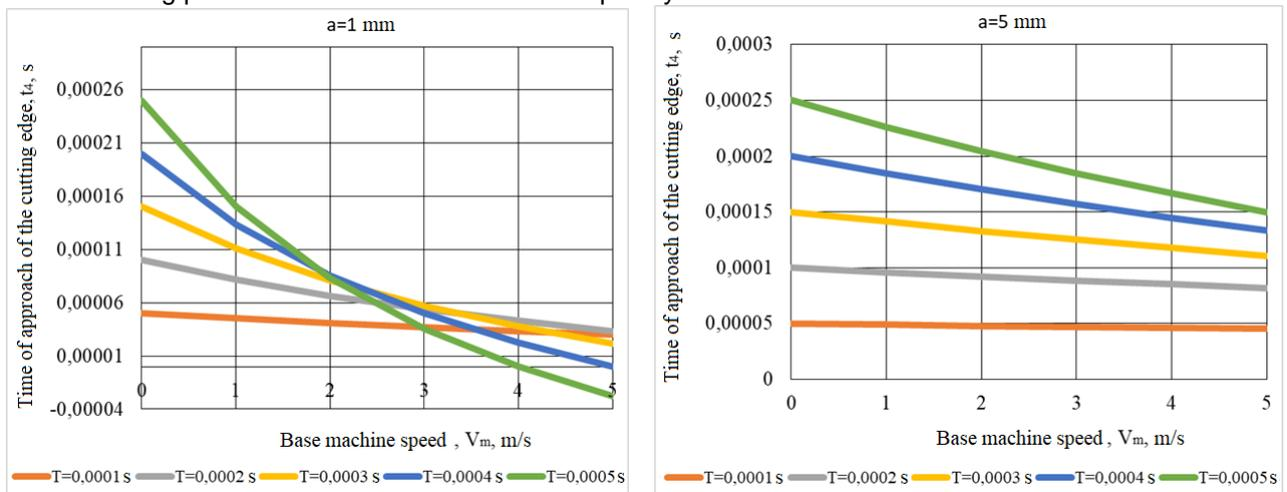
Fig. 8. Influence of the base chassis speed  $V_m$  on time  $t_4$
