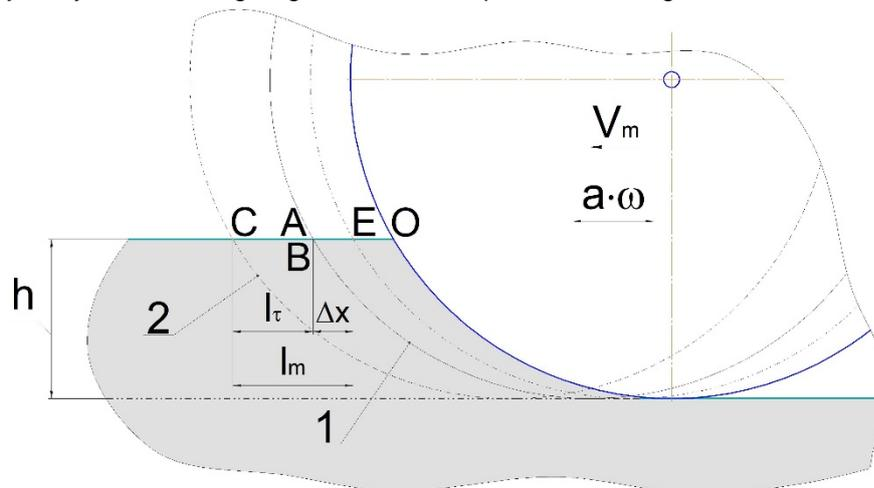
Fig. 3. Diagram of the vibrational cutting process with horizontal oscillations of the tool
