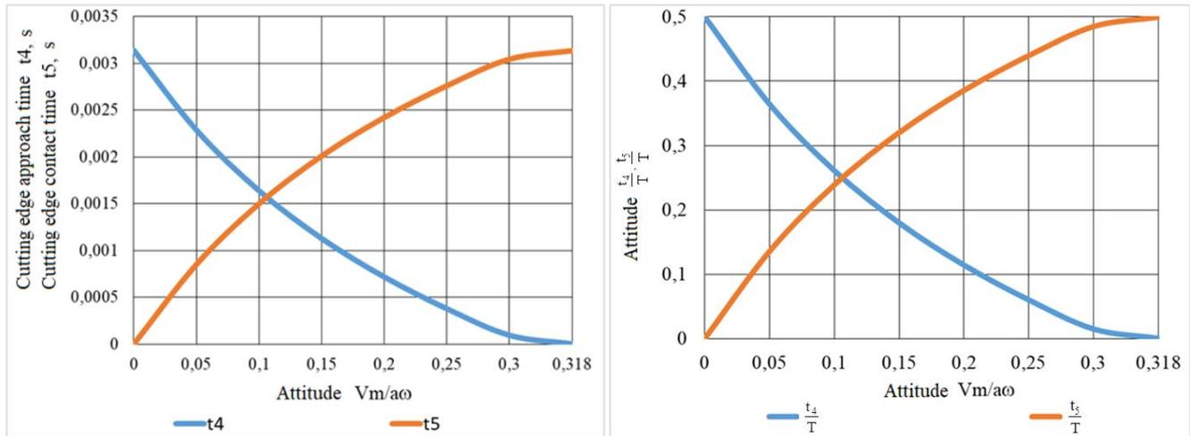
Fig. 10. Influence of the parameter  $\frac{V_m}{a \cdot \omega}$  on the time  $t_4$  and  $t_5$  and on the ratios  $\frac{t_4}{T}$  and  $\frac{t_5}{T}$
