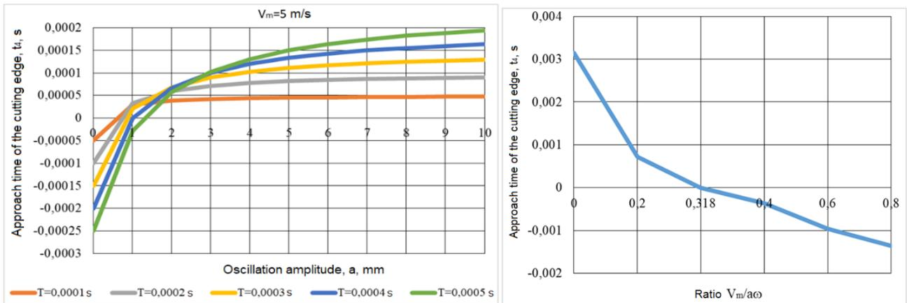
Fig. 7. Influence of oscillation amplitude and parameter  $\frac{V_m}{a \cdot \omega}$  on time  $t_4$
