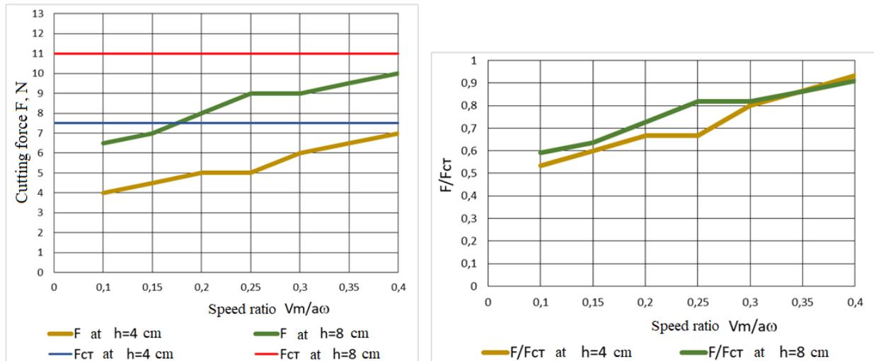
$F_{CT}$  - static soil cutting force;  $F$  - cutting force with a vibrating cutting tool;  $V_m$  - translational speed;  $a, \omega$  - amplitude and frequency of oscillations.
