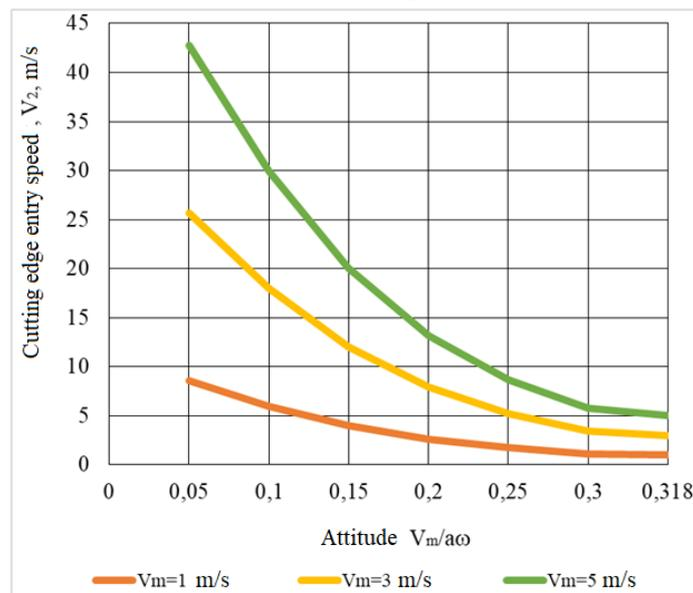
Fig. 9. Influence of the ratio on the penetration velocity of the cutting edge
