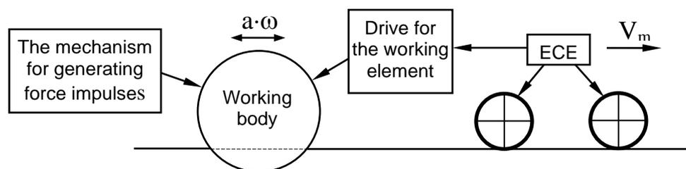
Fig. 2. Structural diagram of a machine with impulse impact on the soil
