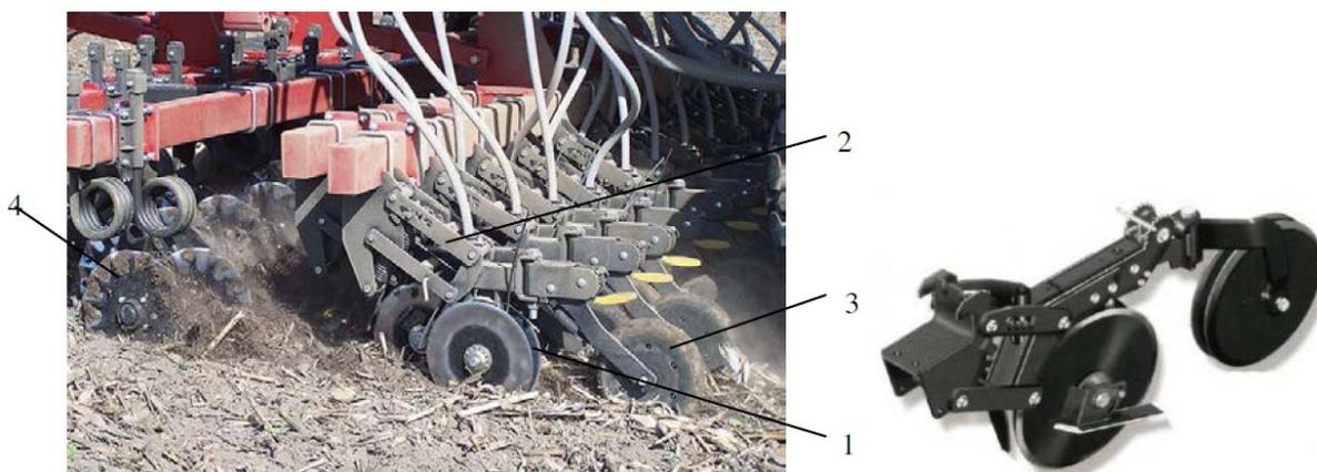
1 - opener; 2 - parallelogram lever mechanism; 3 - roller; 4-disc knife
