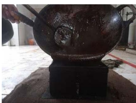
h. Pouring the mixture into a mould
