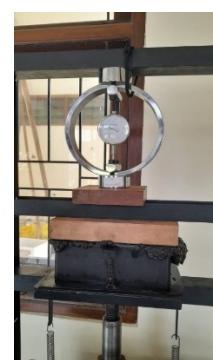
i. Compressing the mixture.
