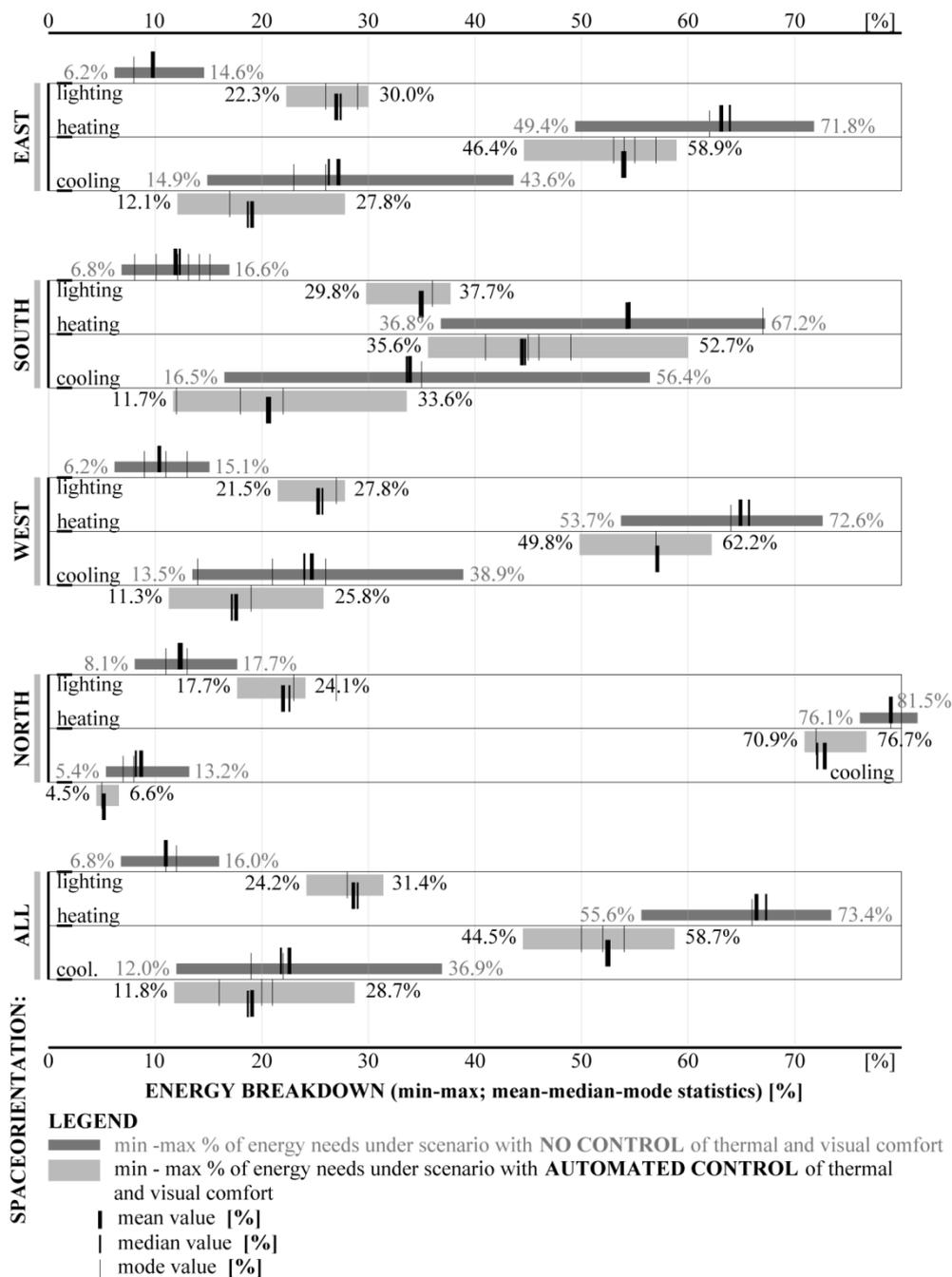
Fig. 2. Results of the study: plotted energy breakdown for simulation runs with and without control of users' visual comfort (plotted data from Table 3)
