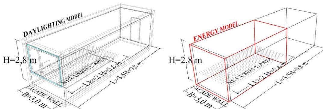
Fig. 1. Daylighting and energy model dimensions and arrangement
