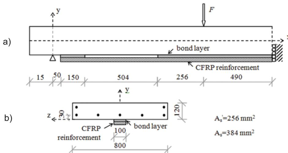
Figure 1. Beam element strengthened with CFRP strip: a) geometry of half beam; b) cross section of the strengthened beam
