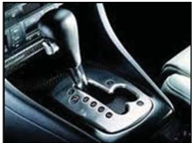
Figure 3: Lever for automatic or manual selection of gears in gear box-Tiptronic [08]
