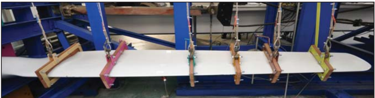
Figure 15: Lyres for the introduction force
