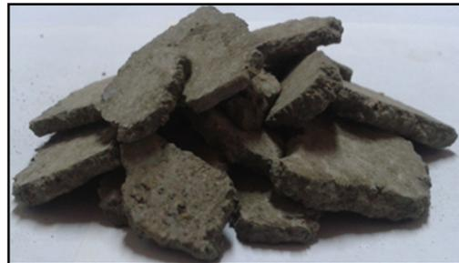
Figure 2. -Klinker after grinding PVI
