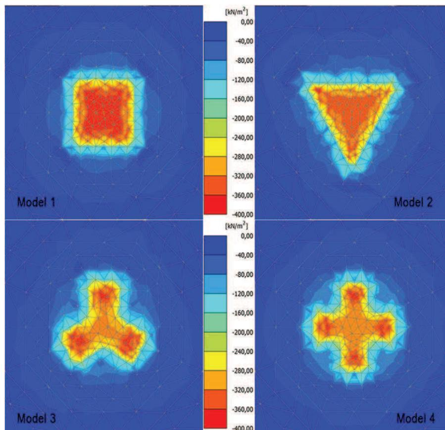
Figure 8: Isolines of vertical stress at the depth of 0,25b in the basis of calculation models of the foundations for cohesive soil at  $P=400$  kPa
