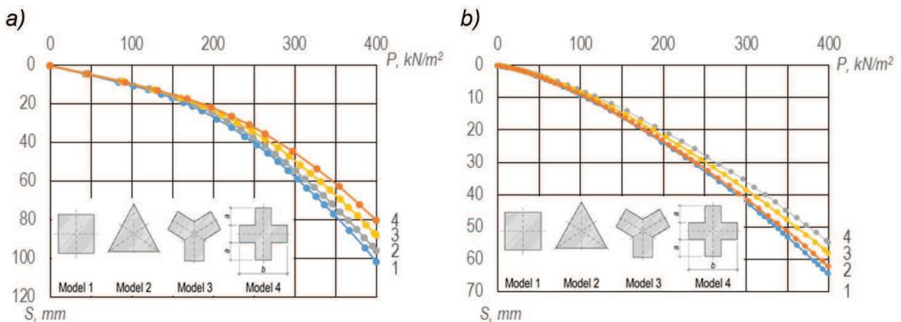
Figure 2: Settlements from vertical loading of  $S=f(P)$  for cohesive (a) and non-cohesive (b) soil with 1 – square; 2 – triangular; 3 – three rayed; 4 – cross-shaped foundations
