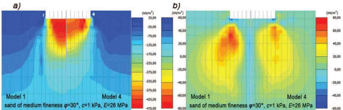
Figure 11: Isolines of vertical (a) and shearing (b) stresses in the basis of square (model 1) and cross-shaped foundations (model 4) at  $P=400$  kPa (non-cohesive soil)
