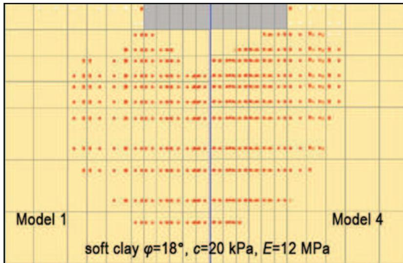
Figure 5: Zones of plastic deformations in the basis of square (model 1) and cross-shaped (model 4) foundations for cohesive soil at  $P=400$  kPa
