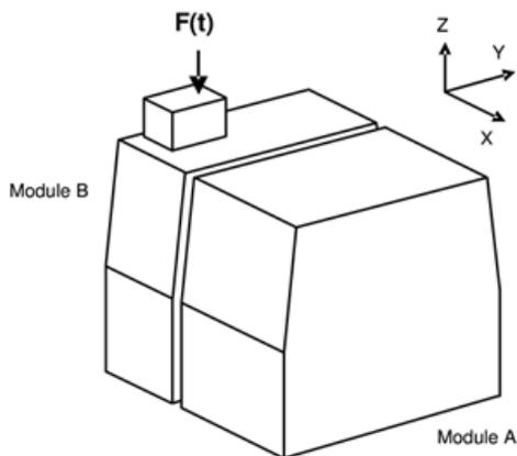
Figure 6e) exciter attached to fixed superstructure in Z direction
