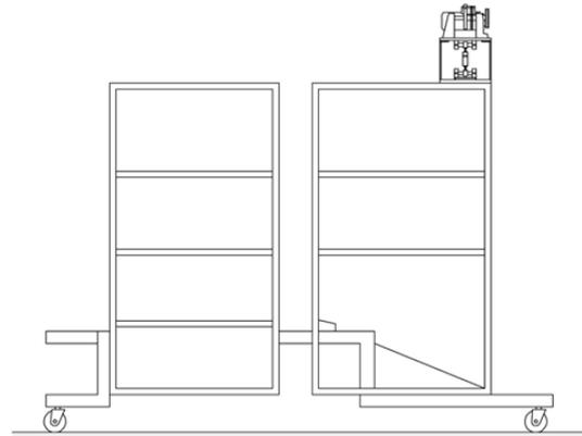
Figure 6h) exciter attached to free superstructure in Z direction
