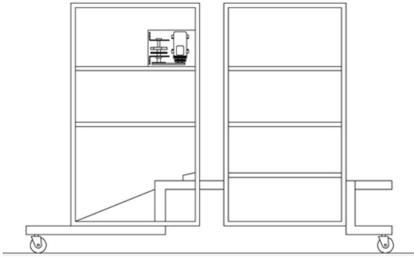
Figure 6g) exciter attached to free superstructure in Y direction
