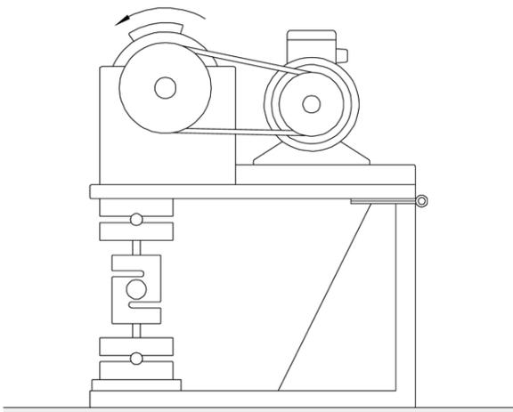
Figure 6a) exciter attached to foundation
