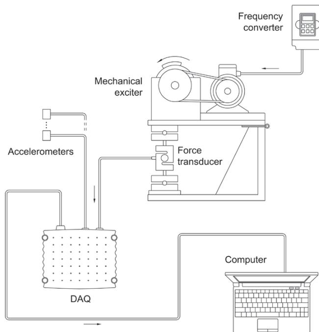
Figure 2. Testing installation
