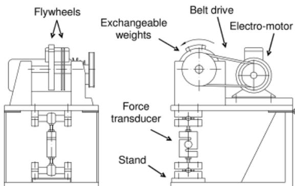
Figure 3. Mechanical vibration exciter
